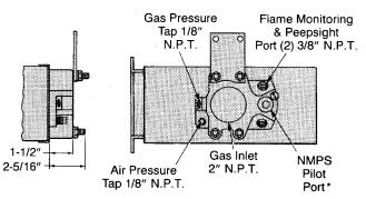
\*On casting #03877-1 for direct spark ignition of 6, 12, & 18 NML burners, this hole is tapped for spark plug #16927.
