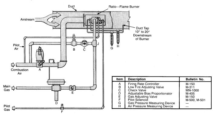
Item "C" stabilizes burner operation at low fire by introducing a partial premix to burner. WARNING: Do not install any value or controlling device in the piping between tee "J" and the burner.
